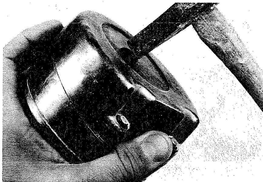
Figure 5:33. Gently Tapping with the Hammer will Separate the Flask Bases from the Molds.
